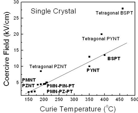
Fig. 4 Coercive field as function of Curie temperature.
