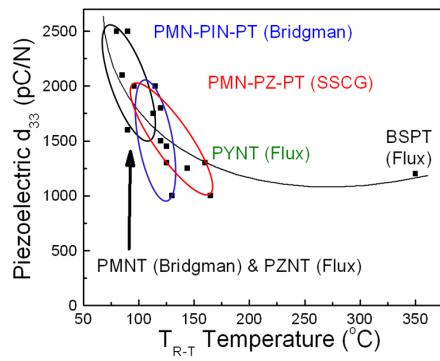
Fig. 3 Piezoelectric coefficients as function of  $T_{RT}$ .
