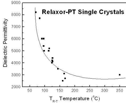
Fig. 2 Dielectric permittivity as function of  $T_{RT}$ .
