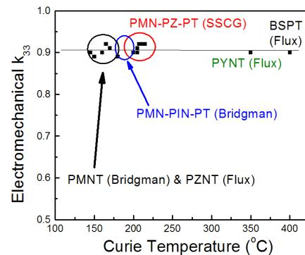
Fig. 1 Electromechanical coupling  $k_{33}$  as function of  $T_c$ .
